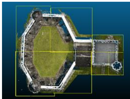
Fig. 3: Model segmented into seven regions for easier processing, with boundaries highlighted in yellow
