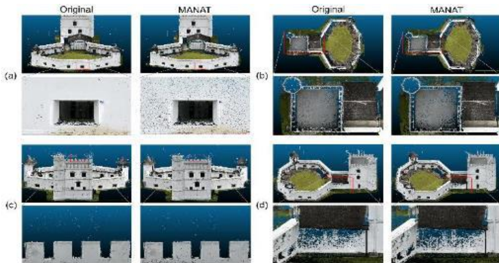
Fig. 6: A visual comparison between the original and MANAT-filtered point clouds across four ROIs. The ROIs include (a) an overview of the fort façade with a zoomed-in view of a window on the perimeter wall, (b) a top-down view of the entire structure with a magnified battlement region, (c) a side view of the fort focusing on the battlements with detailed views of the merlons and crenels, and (d) an oblique view highlighting a wall section beneath the roof
