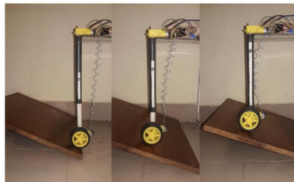
Fig. 8: Testing the robot for different angle surfaces
