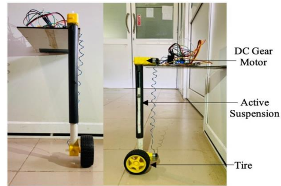
Fig. 3: The formation of the active suspension system. (Quarter-vehicle model)
